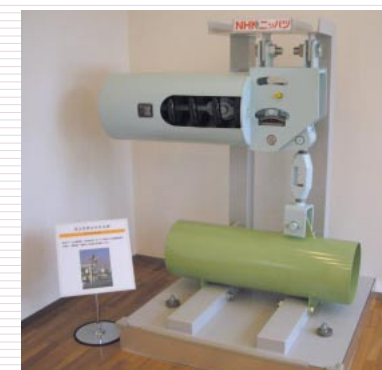
Constant hanger to support pipes under constant loads
