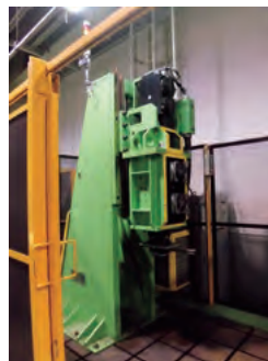
Electric servomechanism fatigue testing machine
