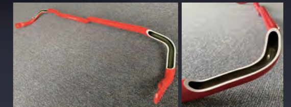
Hollow stabilizer bars Meeting the need for weight reduction, an essential factor in improving fuel efficiency, with processing technology that uses high-strength hollow tubes
